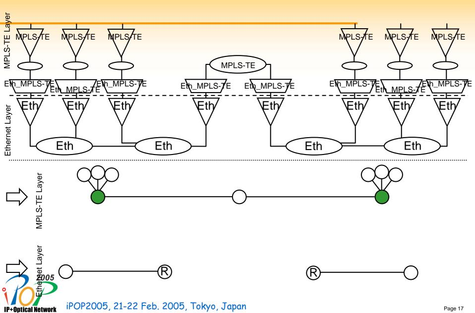
MPLS-TE Routing protocols (e.g. OSPF-TE/ISIS-TE) used for MPLS-TE and Ethernet network routing
