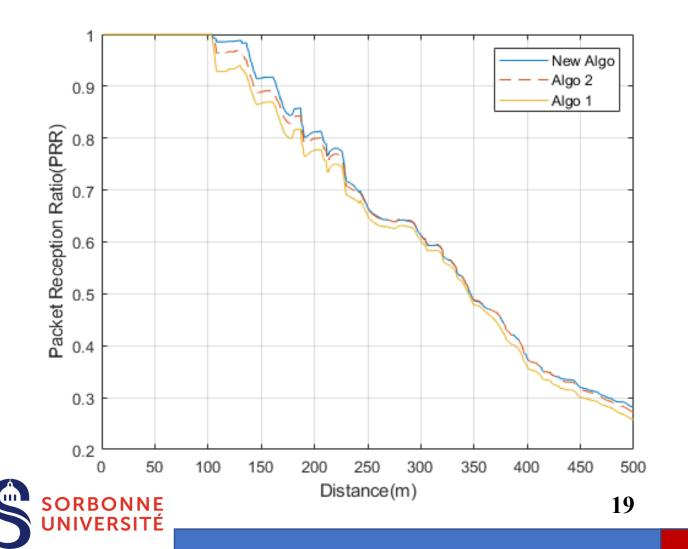
□ The PRR decreases with the increase of the distance between transmitter and receiver.
