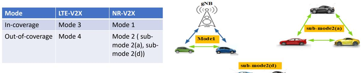
Sub-mode 2(a): UE autonomously selects side-link resources for its transmission
