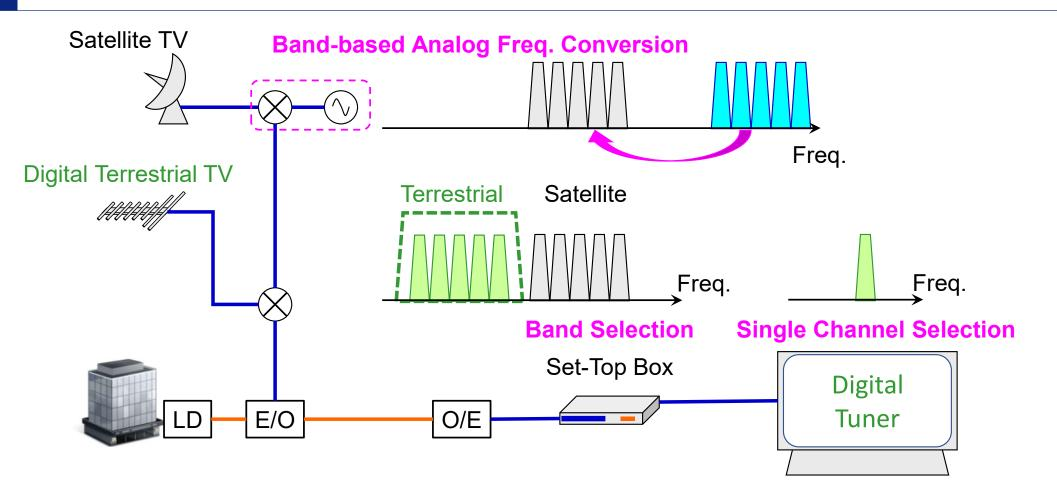
**Band-based Analog Processing + Channel by Channel Digital Processing**
